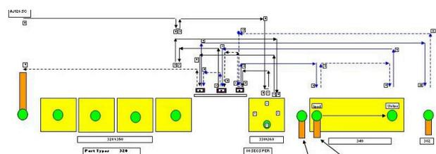
**Figure 1:** Schematic of manufacturing line and gantry movements.
